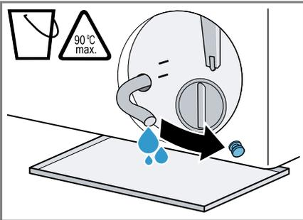
8. Firmly press on the sealing cap.
