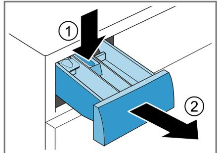
3. Pull out the insert upwards.
