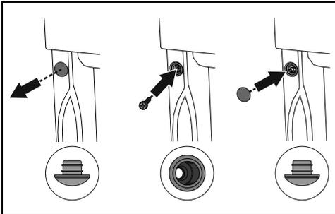
1. Remove the bushing covers on the front of the appliance.
