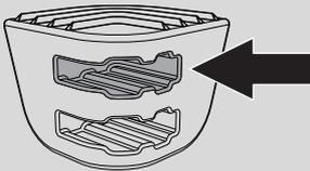
10. Be sure to fit the 4 pins of the inner glass well into their seats on the door.
