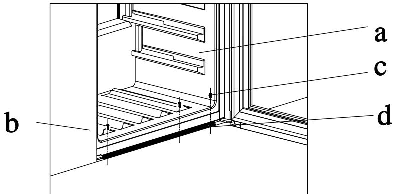
1. Install the wine cooler (a) into cabinet (b) in correct position
