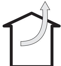
In the extractor mode air is discharged to the outside by a special conduit. In that case any factory-installed charcoal filters shall be removed.
