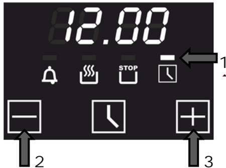
Symbol 1 will start flashing when the unit is switched on for the first time.
