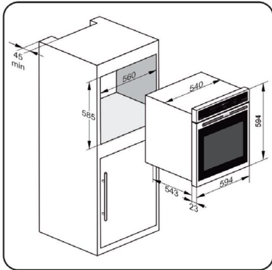
The installation space measurements are given in **mm**.
