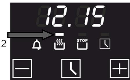
After the end of the countdown the oven emits the triple sound signals with the interval of 2 seconds during two minutes to inform you that all processes in the oven are switched off. The symbol 2 will continue to flash after the end of emitting the sound signals.
