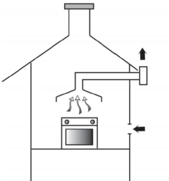
If an electric extractor fan for the removal of foul air is installed in the room, the apertures provided for air changes must allow a ventilation rate of at least 35 m<sup>3</sup>/h per kW of power installed.
