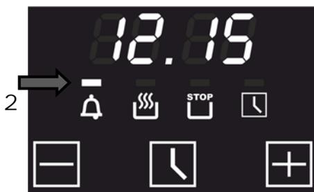
After a few seconds the timer starts the countdown, the display shows the countdown time, the symbol countdown timer 2 appears. By pressing the button 1 you can call up the current time indication for 5 seconds.
