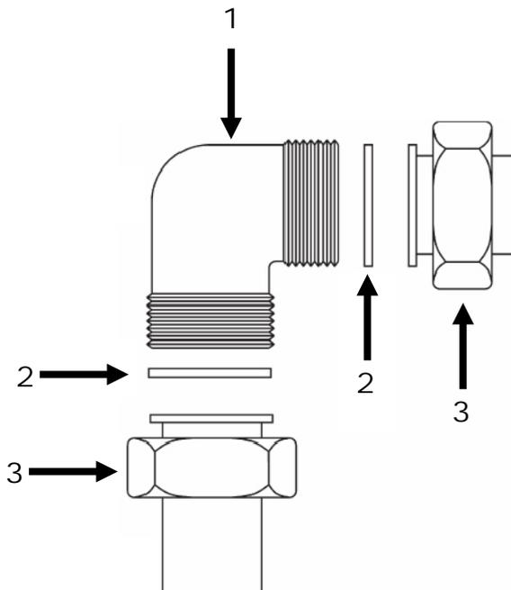
The fitting 1 and seal 2 are supplied with the appliance, and comply with standards.
