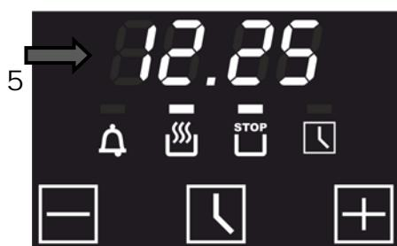
In our example the oven should be turned on at **12:25** (5) with the functions “Grill + Thermocirculation” and be turned off at **12:55** according to your setting.
