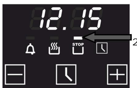
The display shows the countdown time, symbol 2 appears on the display to confirm the successful setting and the current time appears again.
