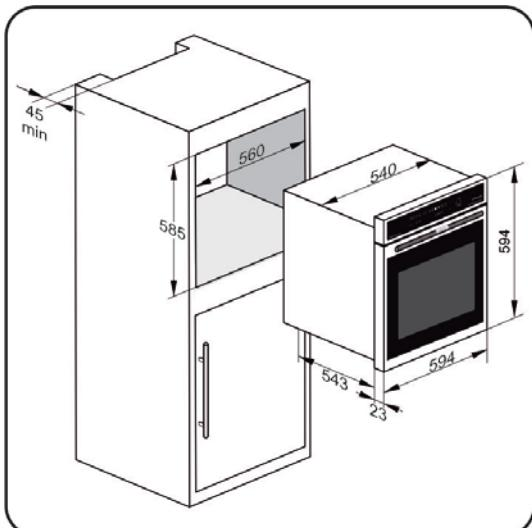
The oven can be installed under a work top or in a cooking column. Figure shows the installation dimensions. Make sure that surrounding materials are heat resistant. Align the oven centrally with respect to the side walls of the units surrounding it and fix it in place with the screws and Allen screws provided.
