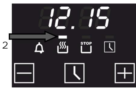
After the end of the countdown the oven emits the triple sound signals with the interval of 2 seconds during two minutes to inform you that all processes in the oven are switched off. The symbol 2 will continue to flash after the end of emitting the sound signals.
