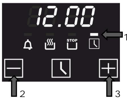
Symbol 1 will start flashing when the unit is switched on for the first time.
